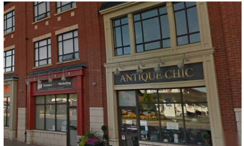
Figure 15 - Front Lit Sign
